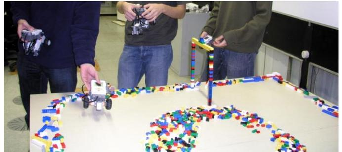
Figure 2. Testing the communication between robots on the racing circuit
