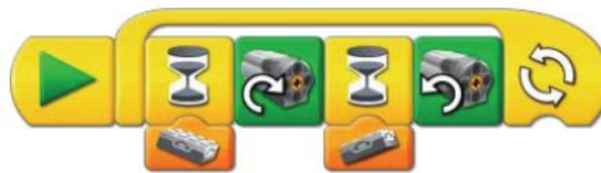
Figure 3. LEGO WeDo kit - simple program that moves the motor according to sensor tilt
